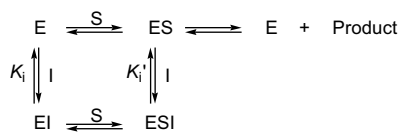
Figure 3. A general model of mixed-type enzyme inhibition. E is the free enzyme, ES is a binary enzyme–substrate complex, EI is the enzyme–inhibitor complex, and ESI is the ternary enzyme–substrate–inhibitor complex.
